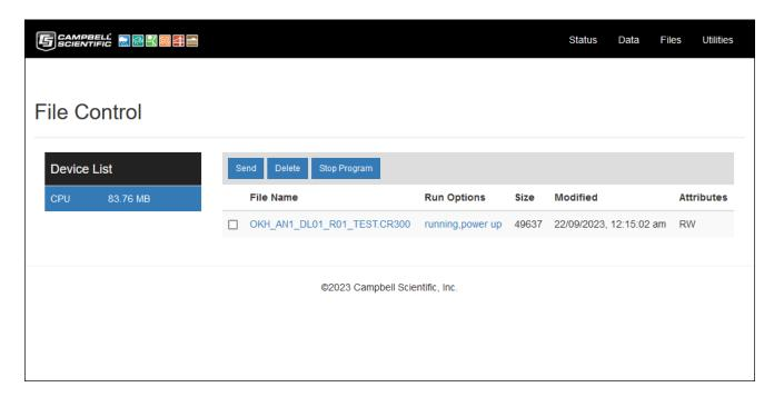
The File Control page enables management of the datalogger files. Files can be sent, deleted, activated, and deactivated. The files page can be selected by clicking on Files on the header/menu bar at the top of the page.
