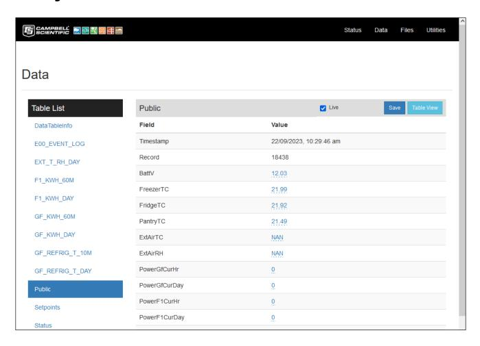
The Data page enables data tables stored in the datalogger to be viewed and downloaded. On some datalogger models this page also allows selected fields to be graphed in realtime. It can be selected by clicking on Data on the header/menu bar at the top of the page.
