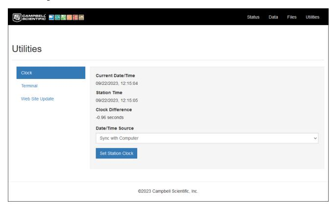
The Utilities page enables setting the datalogger realtime clock and it provides a terminal function. It can be selected by clicking on Utilities on the header/menu bar at the top of the page.
