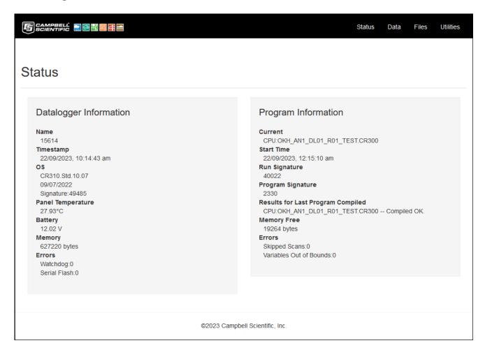
The Status page gives key information about the datalogger and the program that is running in the datalogger. It can be selected by clicking on Status on the header/menu bar at the top of the page.
