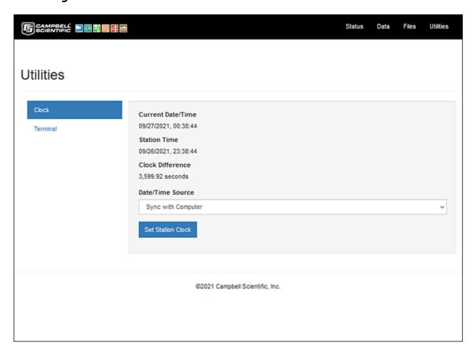
The Utilities page enables setting the datalogger realtime clock and it provides a terminal function. It can be selected by clicking on Utilities on the header/menu bar at the top of the page.
