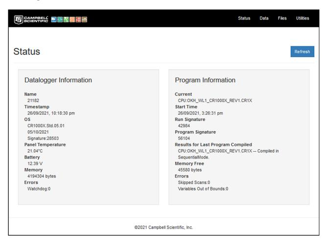
The Status page gives key information about the datalogger and the program that is running in the datalogger. It can be selected by clicking on Status on the header/menu bar at the top of the page.
