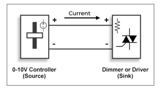
ESTA E1.3 specifies that controllers must be able to source a minimum of 2 mA., It further specifies that dimmers or drivers must have a nominal input impedance of 100K Ohms. This means that a fully compliant dimmer should only draw only about 0.1 mA from the controller when the control voltage is set at 10V which allows several dimmers or drivers to be connected to a single controller channel.
