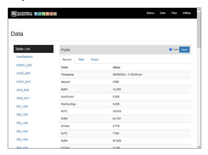
The Data page enables data tables stored in the datalogger to be viewed and downloaded, or selected fields graphed in realtime. It can be selected by clicking on Data on the header/menu bar at the top of the page.
