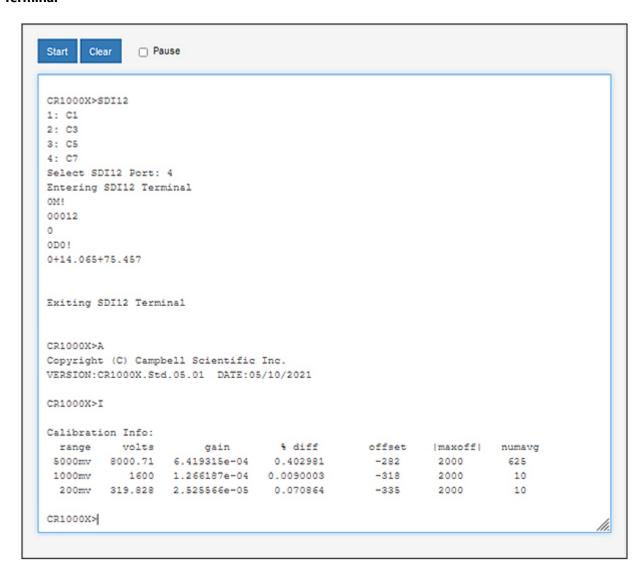
The terminal function is primarily an engineering tool. It is not necessary to use it for routine datalogger operations other than configuring SDI-12 sensors. A sample Terminal session is shown below.
