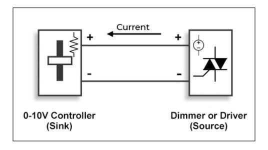
IEC 60929 Annex E specifies that the control current must not exceed 2 mA. Given that most LED drivers only require a fraction of that current, several LED drivers can usually be connected to a single controller channel.
