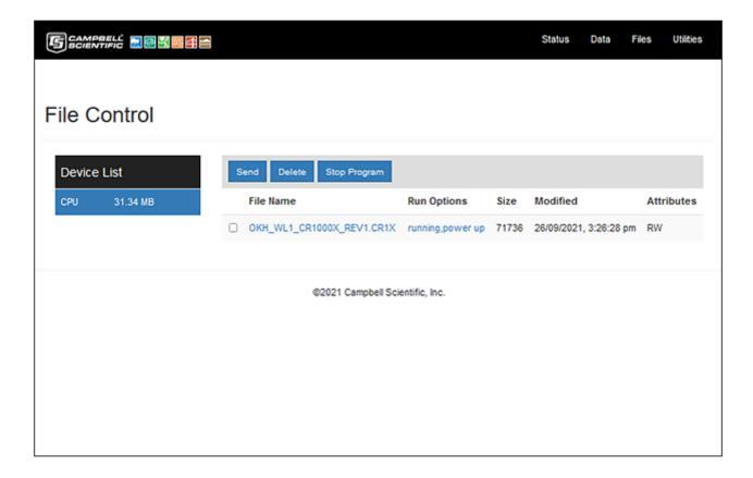
The File Control page enables management of the datalogger files. Files can be sent, deleted, activated, and deactivated. It can be selected by clicking on Files on the header/menu bar at the top of the page.
