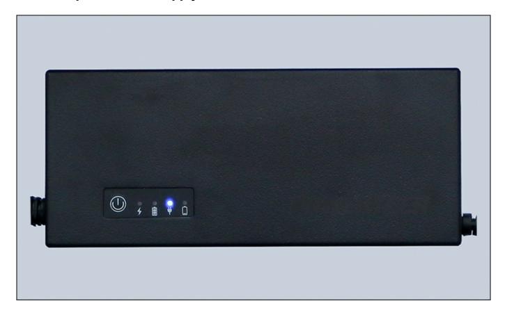
An uninterruptible power supply (UPS) ensures the datalogger continues to record data and transmit alarms during power failure events. The UPS is a DC-DC type, with an integral lithium-ion rechargeable battery. Its input is 12 Vdc, which comes from a mains powered power supply, and its output is 12 Vdc, which is used to power the datalogger and control system.
